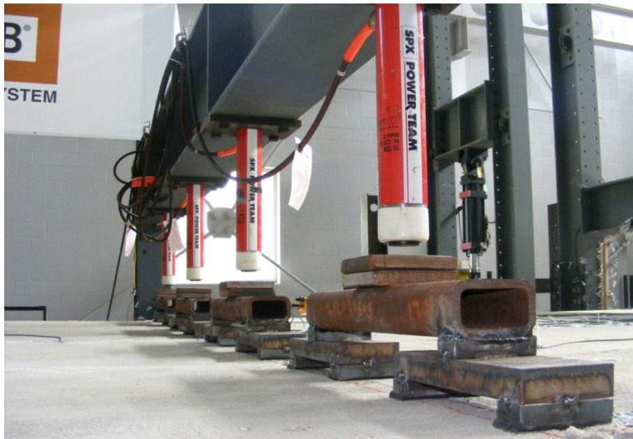
Figure 2: Hydraulic loading cylinders and load distribution elements
