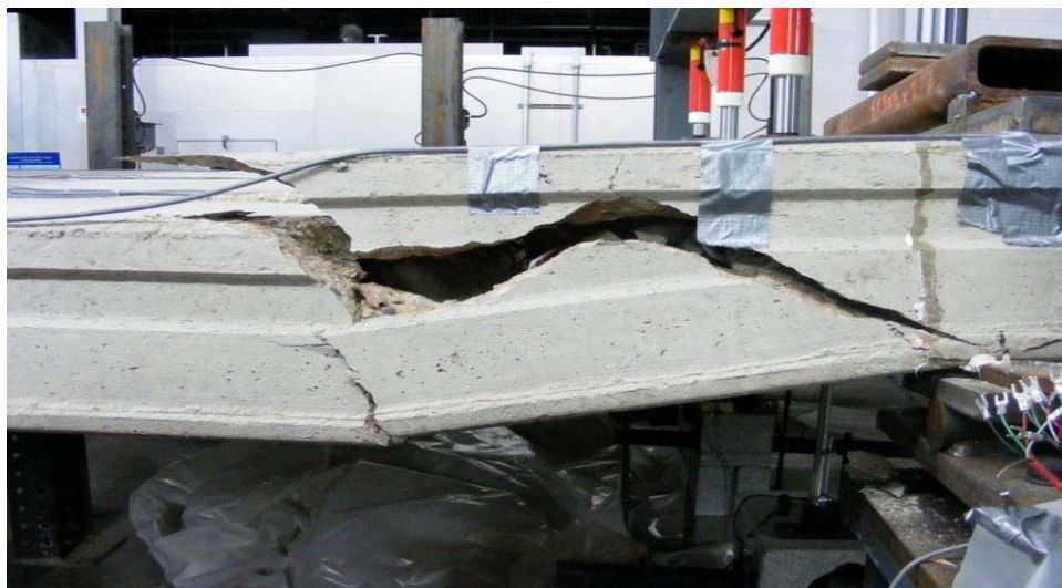
Figure 6: Test was stopped after severe distortion of slab due to shear cracking
