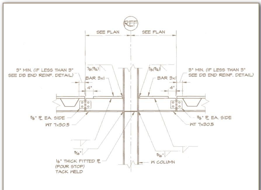
Detail of column “goosenecks”—beam “stubs” moment-connected to the columns to reduce the effective span of the girders.
